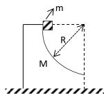
A small cube of mass m slides down a circular path of radius R cut into a large block of mass M as shown. M rests on a table and both blocks move without friction. The blocks are initially rest and m starts from the top of the path.
